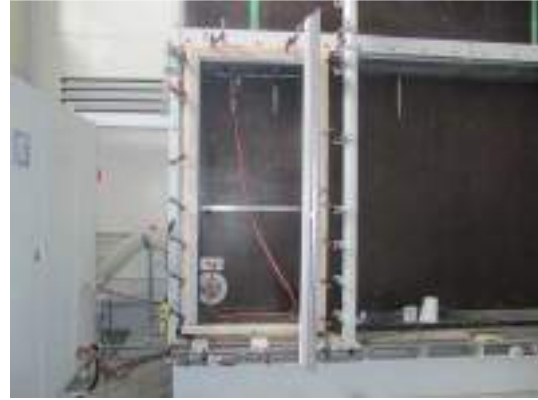
Photo 2 View of test specimen on window test rig Window open
