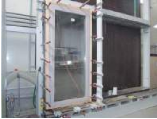
Photo 1 View of test specimen on window test rig Window closed
