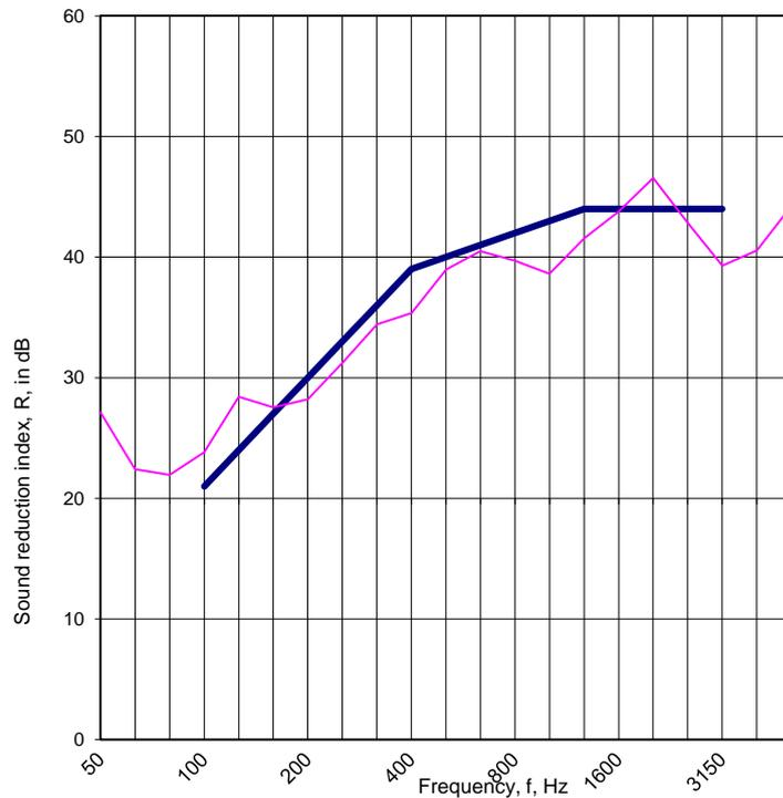
— Rating Curve (ISO 717-1)    — Sound Reduction Index, R, in dB
